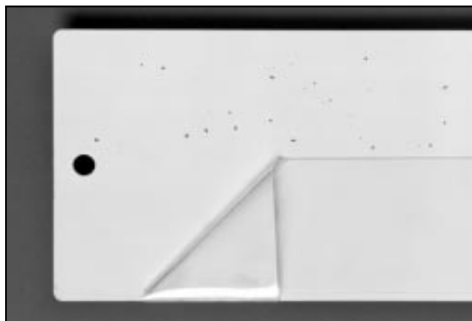
This painted panel subjected to a rugged gravelometer test shows the protective benefit of using 3M™ Scotchcal™ Paint Protection Film.
